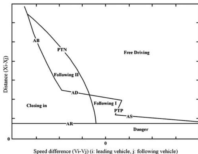
**Figure 3** Fritzsche car-following diagram (After Fritzsche, 1994).
