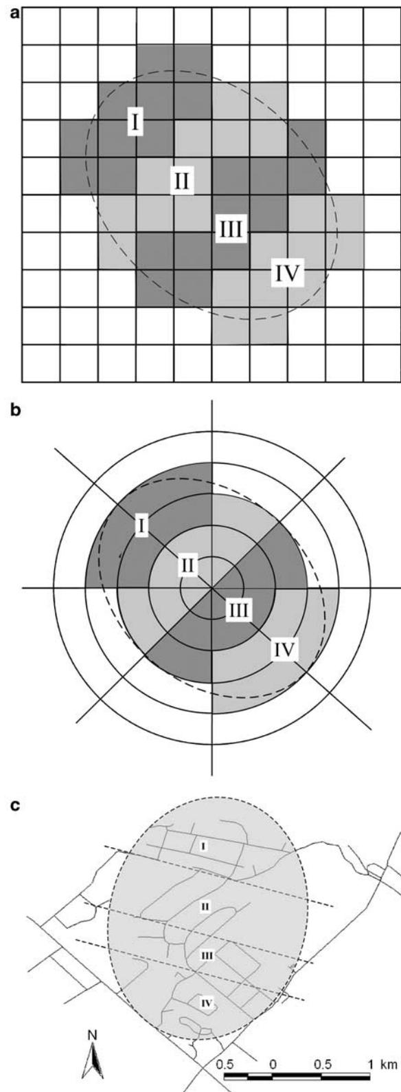
**Figure 1** Simulated road networks used in the simulation and the division of the four zones in the affected area: (a) grid road network, (b) ring road network, (c) real road network. (Note: ellipse—hypothetical affected area, solid lines—road networks, dashed lines in (c)—zone divisions).
