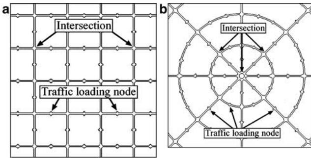
**Figure 2** Examples of traffic loading positions: (a) grid road network, (b) ring road network.
